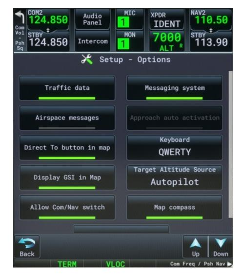
The COM/NAV buttons display the current index (here COM2/NAV2).
