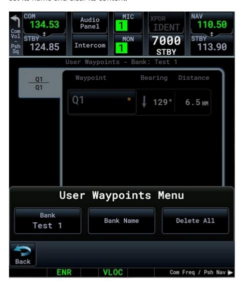
You can insert user waypoints from different banks to the flight plan.
