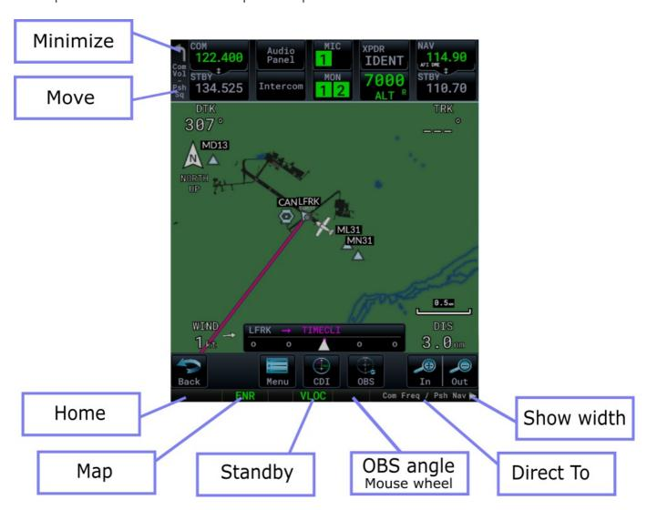
The OBS Angle is available only when the current page is the map. Use the mouse wheel to change the angle. You can also click the OBS indicator to enter the OBS value directly. The Show width button will help you to resize the panel.
