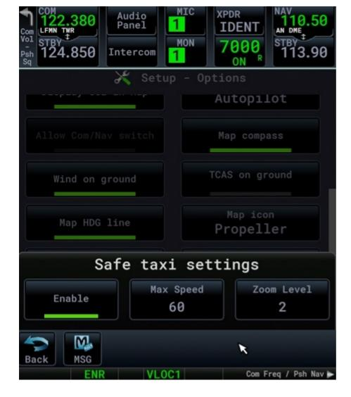
The "Max Speed" parameter indicates the maximum speed below which the system will be engaged after landing (default 50kts).
