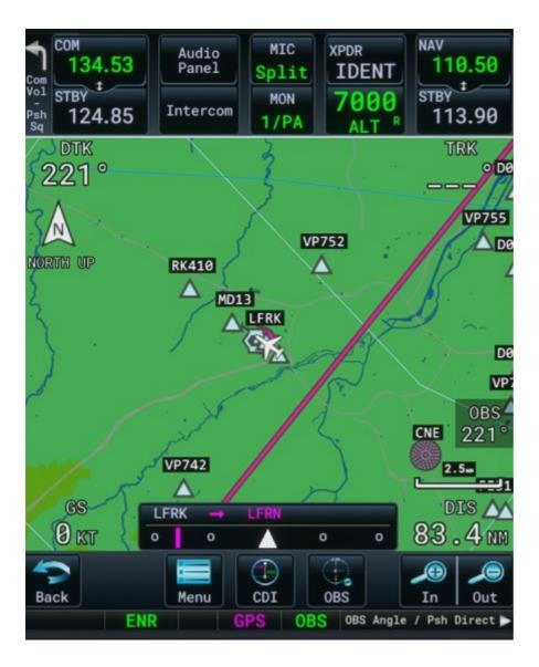
Pushing the knob restores the OBS angle to the initial desired track.
