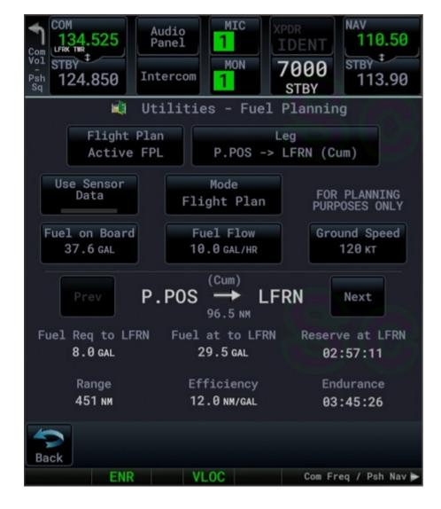
To refresh the leg list while in flight plan mode, press the Flight plan key. Press the menu button to set fuel type and unit.
