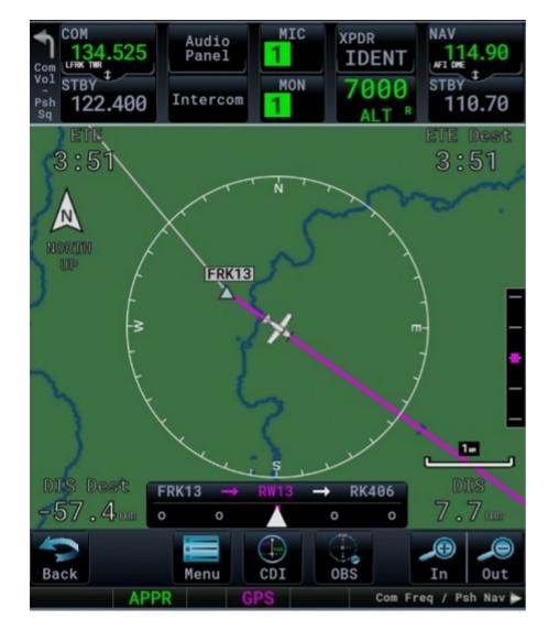
With a WTT compatible airplane the GSI is also displayed for visual approaches.
