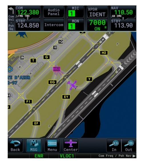
When enabled, the main map page automatically switches to the utility map page after landing and shows you the detailed airport map with the airplane position. There is currently no traffic data displayed.
