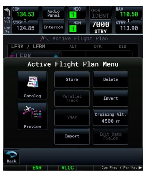
Changing the cruising altitude will update the altitude of all the enroute waypoints. Any entered cruising altitude less than 1000ft will reset the cruising altitude. The cruising altitude is limited to 20000 feet (sim limitation).
